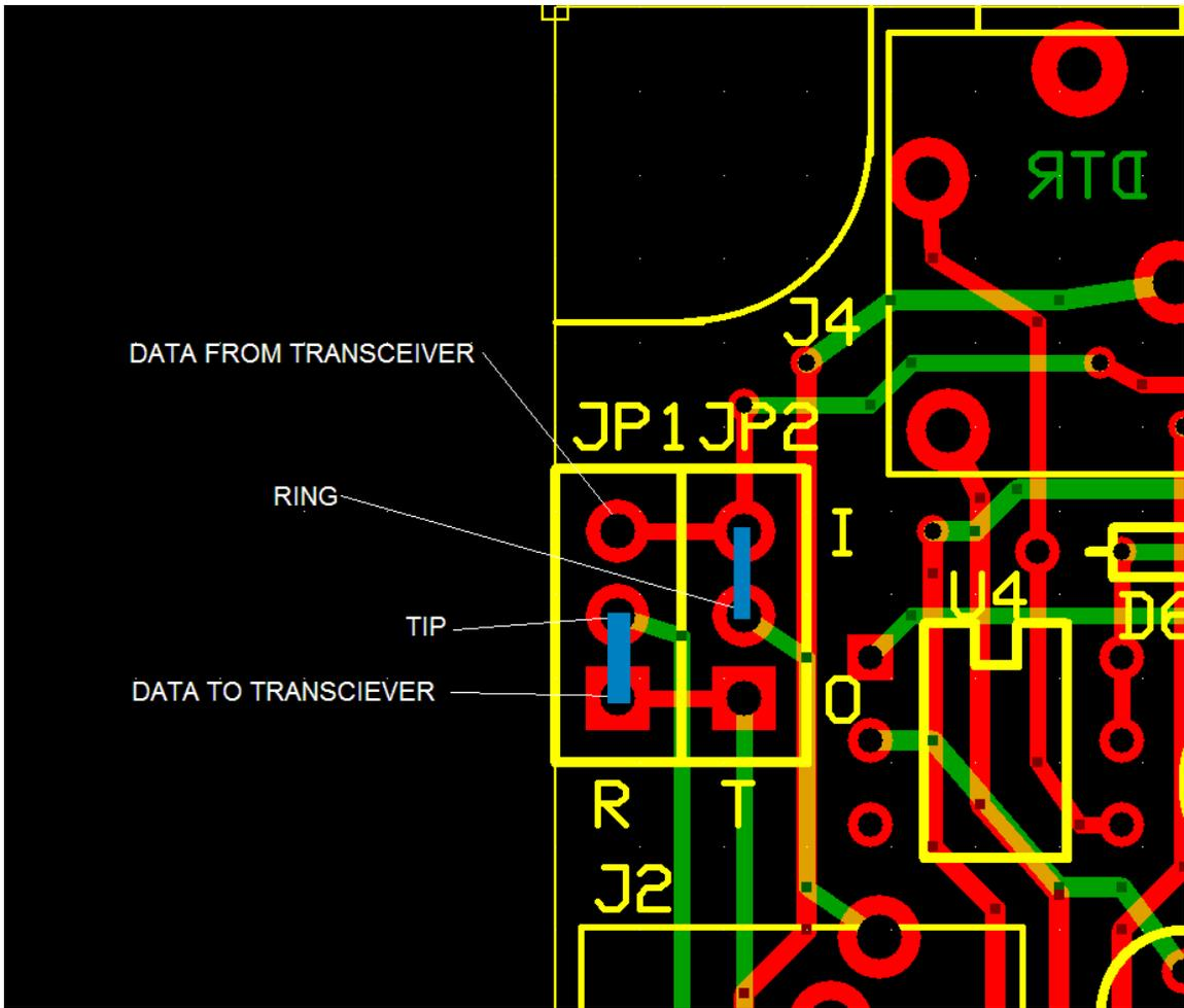
Install jumpers as shown to place the signal from the transceiver to the IsoCat on the ring and the data signals from the IsoCat to the transceiver on the tip. Ground remains the same. Wire the opposite end of the cable to the appropriate pins on the connector required by your transceiver.
